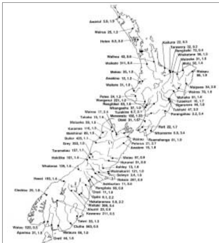
Fig. 3 Mean flows ( m^3/s ) and coefficients of variation of major New Zealand rivers (from Duncan 1992).
